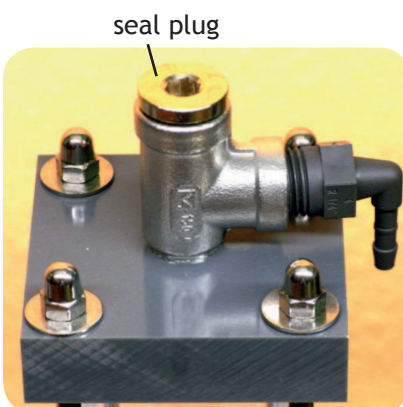
If no pressure gauge available: Screw seal plug into upper outlet of T-pipe (gasket enclosed with plug).
