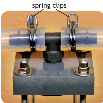
Cut thick hose (from Accessories Set) into halves. Tighten with spring clips to the double sided hose connector.
